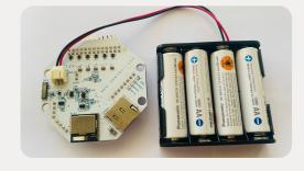
Loop the battery pack's cable through the hole on the other piece of the case then plug in the 6V AA battery pack to Cython board.
