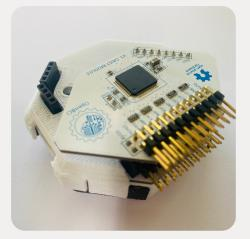
Attach the Daisy extension on top of the Cyton Board with the case in between.
