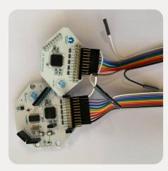
Use the HPTA cables to connect bottom pins N1P - N8P of Cyton board and Daisy to the cables of the EEG cap.
