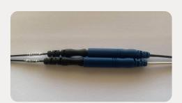
Connect the single end of the Y-Splitter to the REF cable of the EEG cap.
