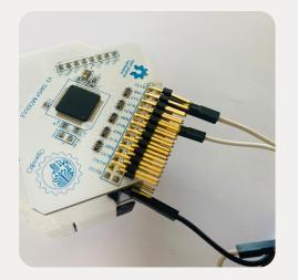
For reference, connect the white Y-Splitter Cable to the bottom SRB pin of the Daisy and Cyton Board.
